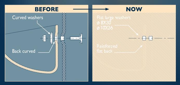
Following this modification, the attachment area of plastic buckets strengthened and efforts are better distributed on the back of the bucket. Flat Washers to use now are 8x30 and 10x36.
